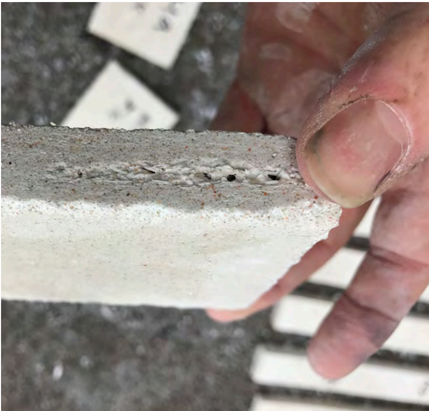
Figure 6 Example of badly compacted GRC
