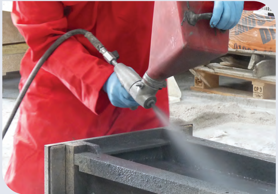
ABOVE: Application of facing coat: hopper gun.
