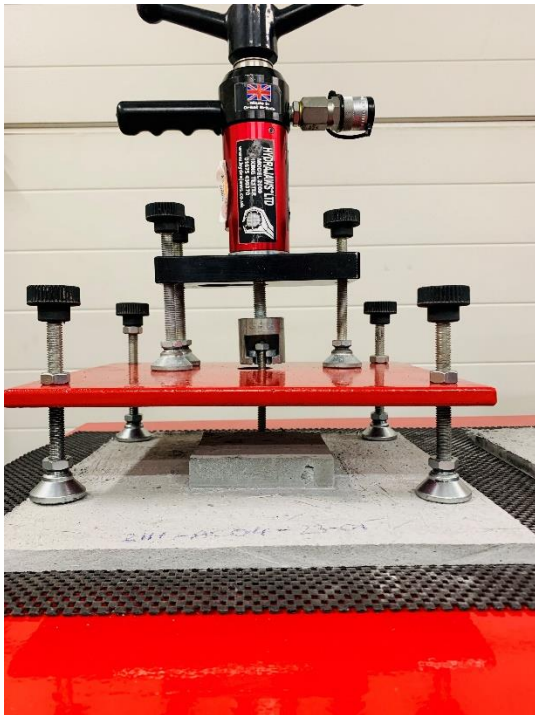
Testing pull-off capacity of anchor pads.
