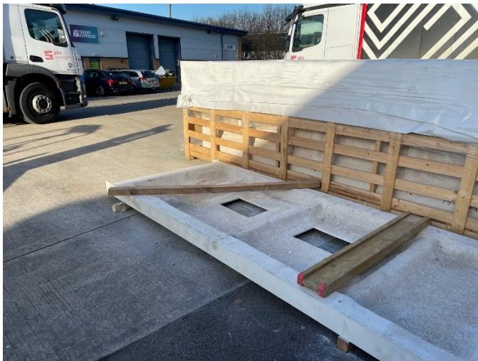
Sampling of full-sized panels for facing coat and flexural testing
