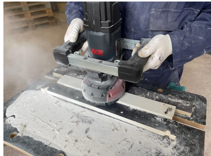
Removal of facing coat to determine thickness and prepare specimen for flexural testing.
