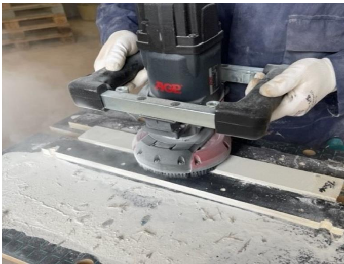
Sample from finished product being tested for facing coat/structural GRC thickness
